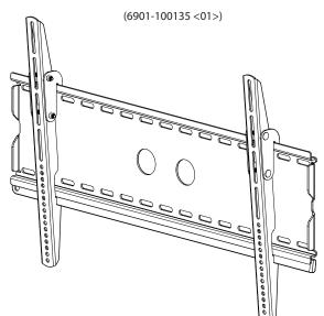
Thank you for choosing the Sanus Systems Vision Mount wall mount. The Sanus Systems VMPL2 wall mount is designed to support a monitor weighing up to 79 kg (175 lbs) to a vertical wall either flat or at a fixed 5 degree tilt. Hardware for multiple mounting configurations is included.
